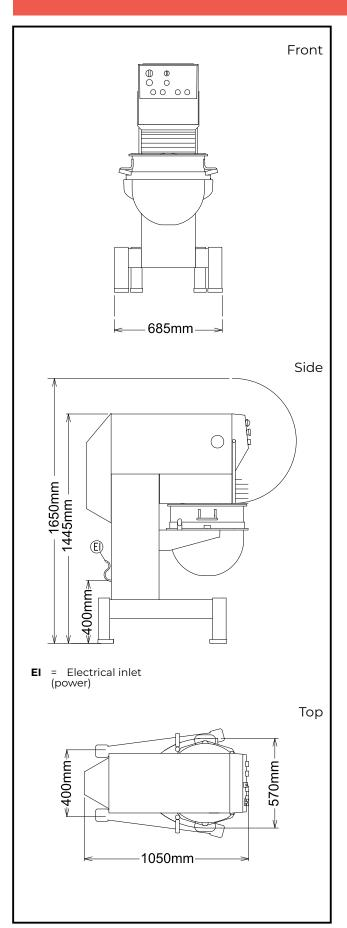
Electric Supply voltage: 380-440 V/3N ph/50/60 Hz 600185 (DXBE60XB3) Electrical power max.: 4 kW **Total Watts:** 4 kW Capacity: ISO 9001; ISO 14001 kg/ Performance (up to): Cycle 60 litres Capacity: Key Information: External dimensions, Width: 685 mm External dimensions. 1050 mm Depth: External dimensions, Height: 1445 mm **Shipping weight:** 306 kg ISO 9001; ISO 14001 kg **Cold water paste:** with Spiral hook
